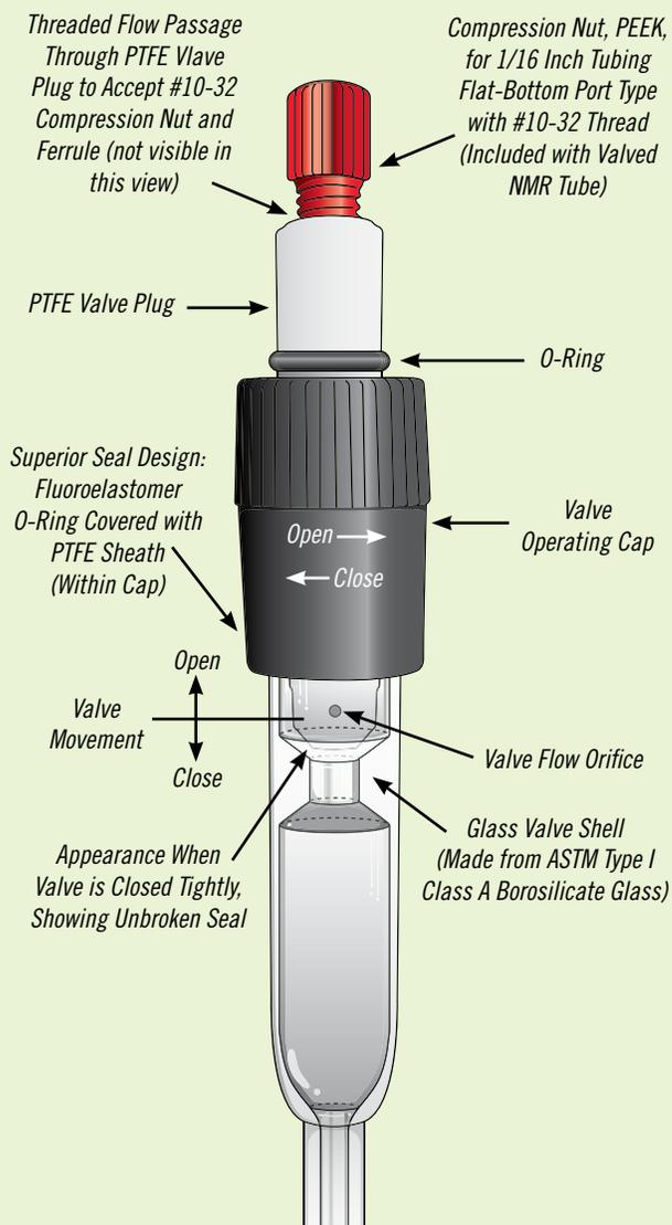
1. To make the connection to a pressure source, such as an argon or hydrogen gas cylinder, for example, one end of a short length of PEEK or PTFE pressure tubing of 1/16 inch OD (not supplied with the IPV Valved NMR Tube) must first be connected to the gas pressure regulator outlet, or other source of gas pressure. (Ensure that the regulated pressure is within the safe limits described above for the particular IPV Valved NMR Tube to be used, as well).
